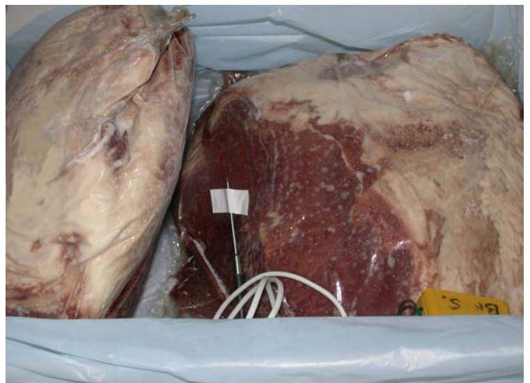
Figure 4: Sensor taped between touching surfaces of primal cuts
