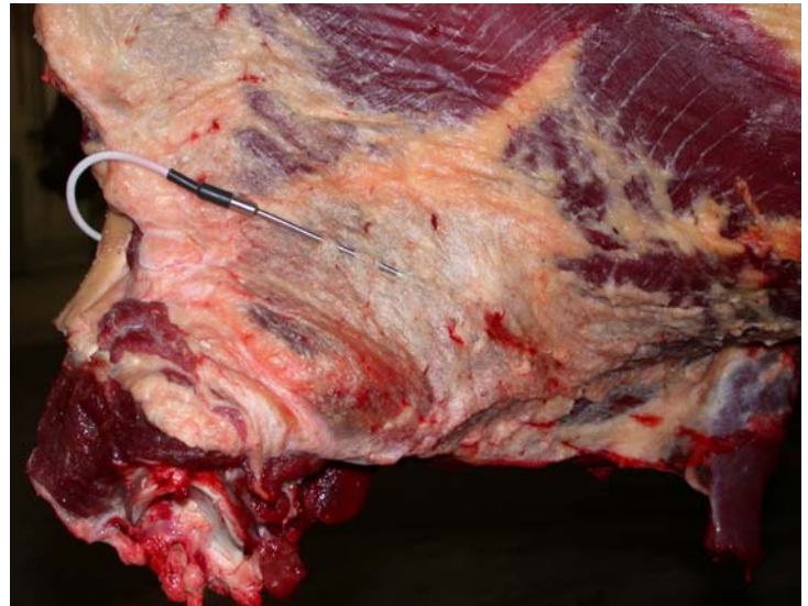
Figure 2: Placement of the temperature probe on the neck of a beef side
