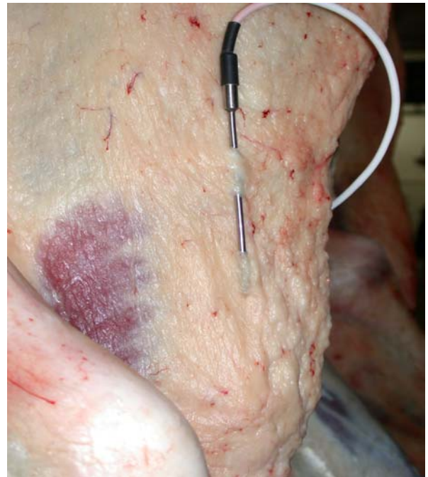
Figure 1: Placement of the temperature probe on the brisket of a beef side.
