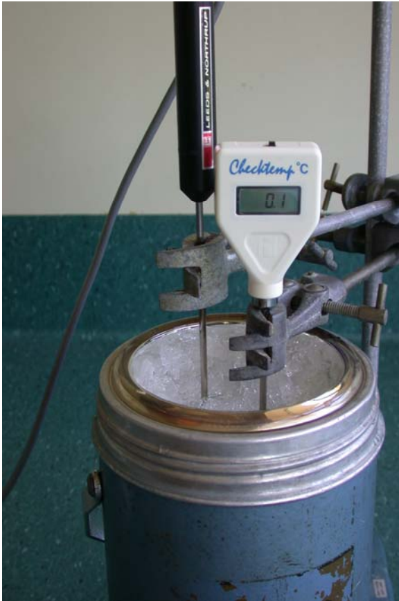
Figure 1: Calibration of working thermometer in ice/water with reference thermometer.
