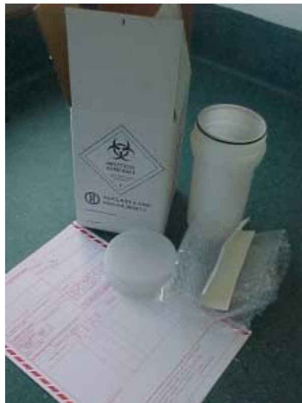
Figure 1. A dangerous goods packing container and declaration form for the transportation of infectious substances.
