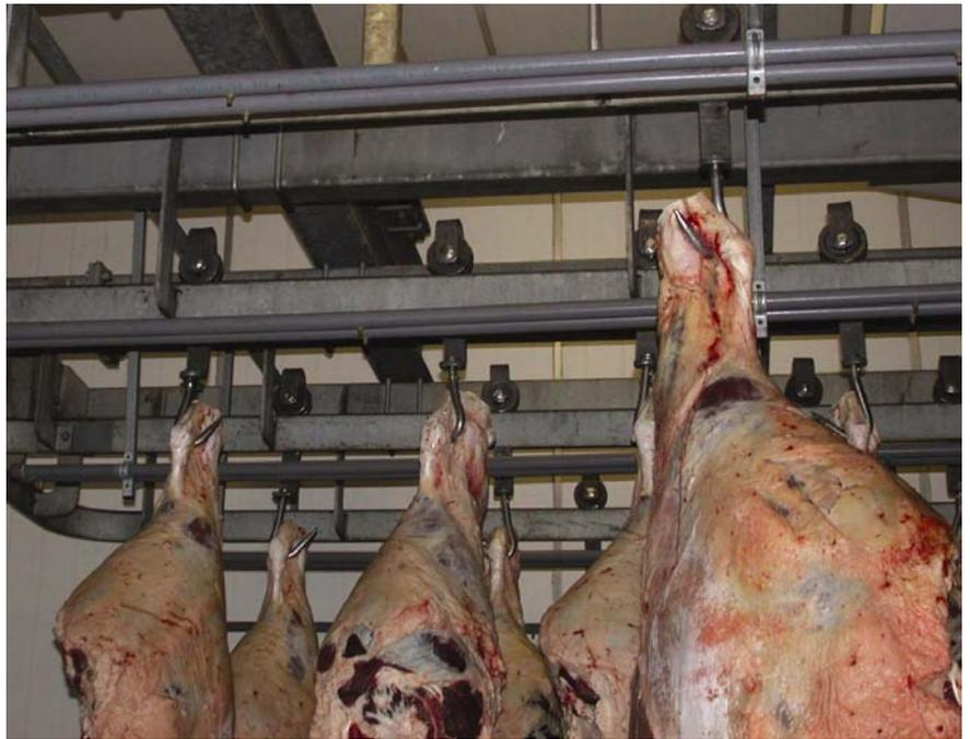
Figure 1. Water lines and spray nozzles positioned above carcasses in chiller.
