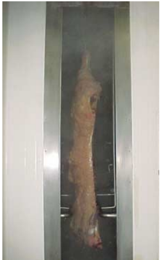
Figure 1. Hot water treatment of beef sides in an Australian abattoir.
