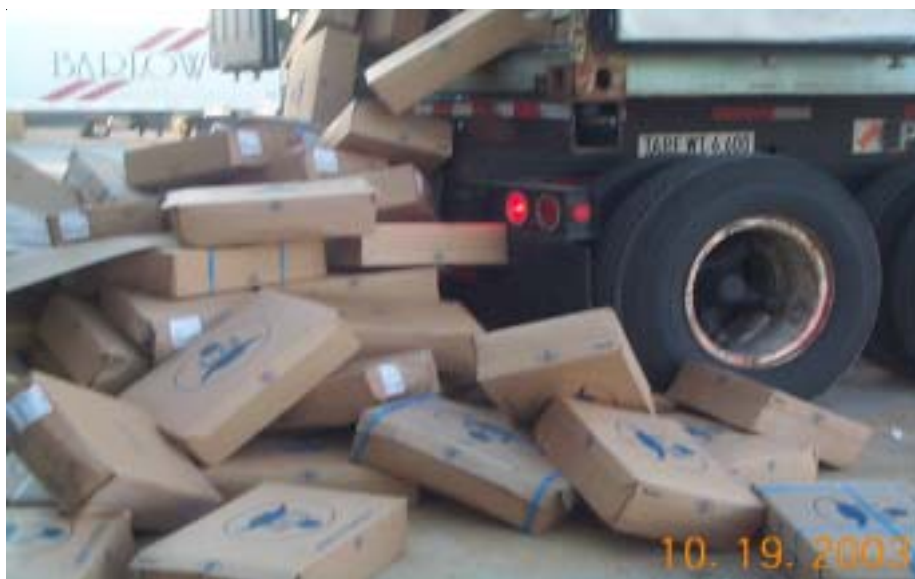
Figure 2: Fallen cartons on opening container doors (courtesy of Mullica Hill Group)
