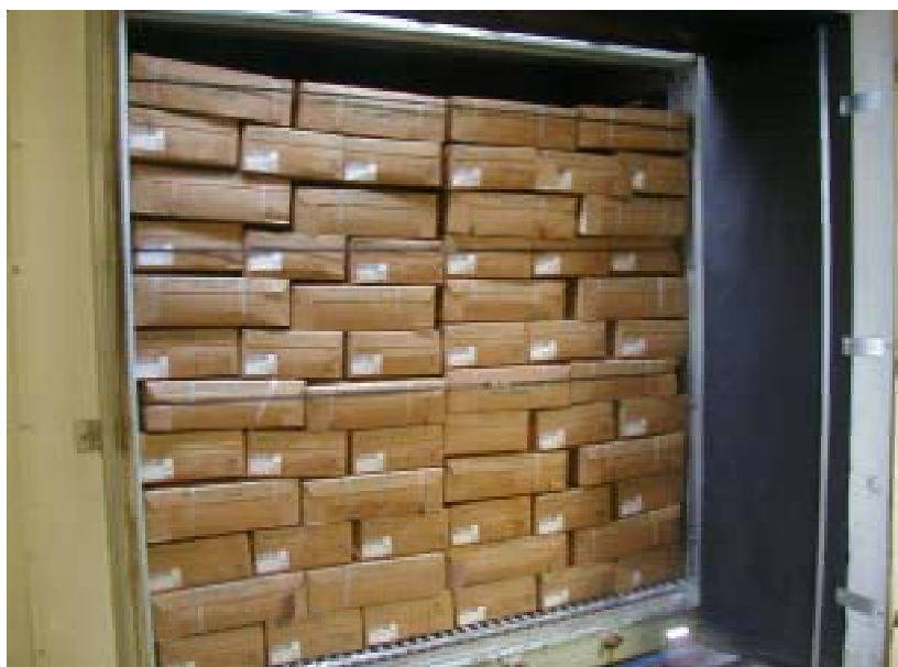
Figure 3: Interlocked stacking and banding technique (courtesy of Mullica Hill Group)
