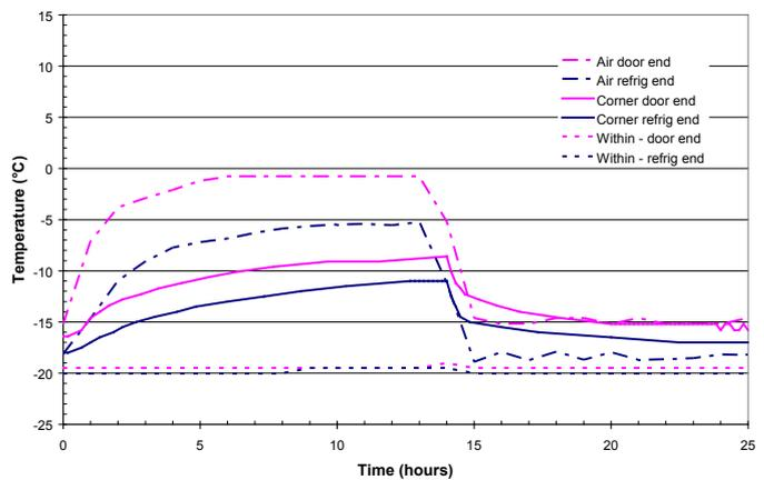
Figure 3: Air and meat surface temperatures in a container off power for 14 hours
