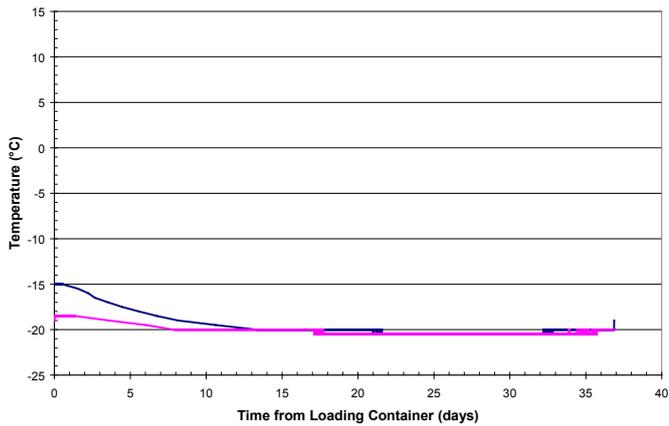
Figure 2: Product loaded into a container above the carriage temperature can take up to 2 weeks to cool.
