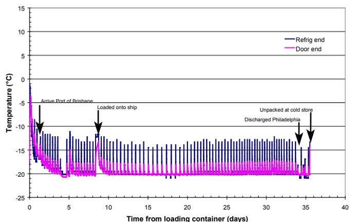
Figure 4: Meat surface temperatures at the top corners of a container
