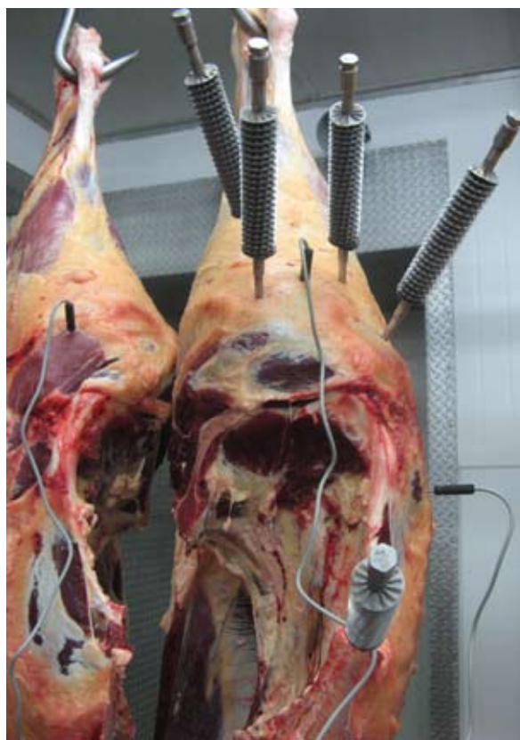
Figure 3: Location of heat pipes and thermocouples for the leg and loin for control and treatment sides. Note: The heat tubes must be placed at an angle above horizontal, in order to work.
