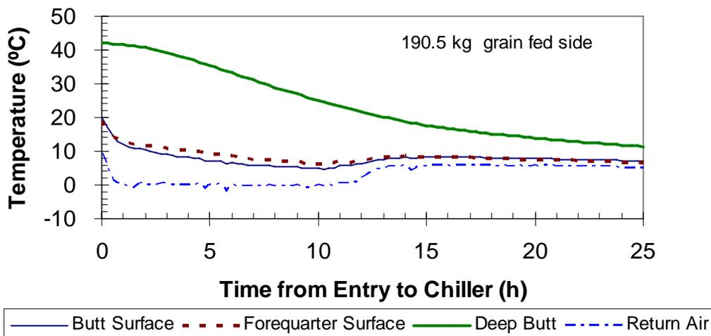
**Figure 1: Typical current chilling cycle for beef sides**
