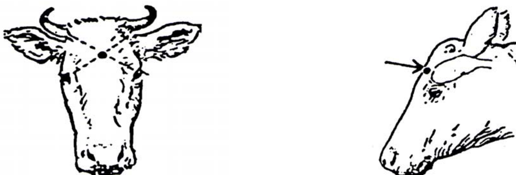
FIGURE 3: The frontal position for application of the stunner
